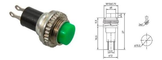
DS-314 10mm diameter momentary ON or momentary OFF mini pushbutton switch Specification: Ambient temperature: -10°C~+85°C Contact resistance: < 20MΩ Insulation resistance: >500VDC 100MΩ Minute Withstand voltage: >1000VAC, 1 Minute Operating Temperature: -25°C~+85°C Mechanical life: >50000 CYCLES Electrical life: >10000 CYCLES
