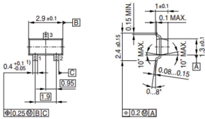
1) Lead width can be 0.6 max. in dambar area
