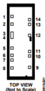
Figure 4. Die (820 μm × 2255 μm)
